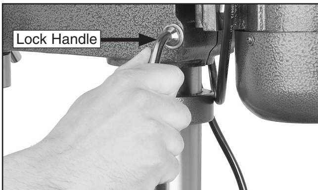
Figure 11. Securing headstock to column.
